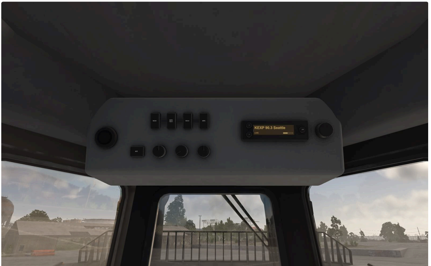
Overhead panel: fan, temperature, air mode, A/C, wipers and radio
