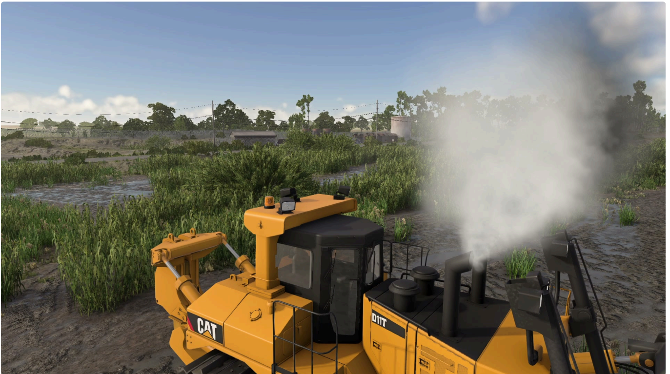
Cold start: white smoke and a rough, hunting idle
