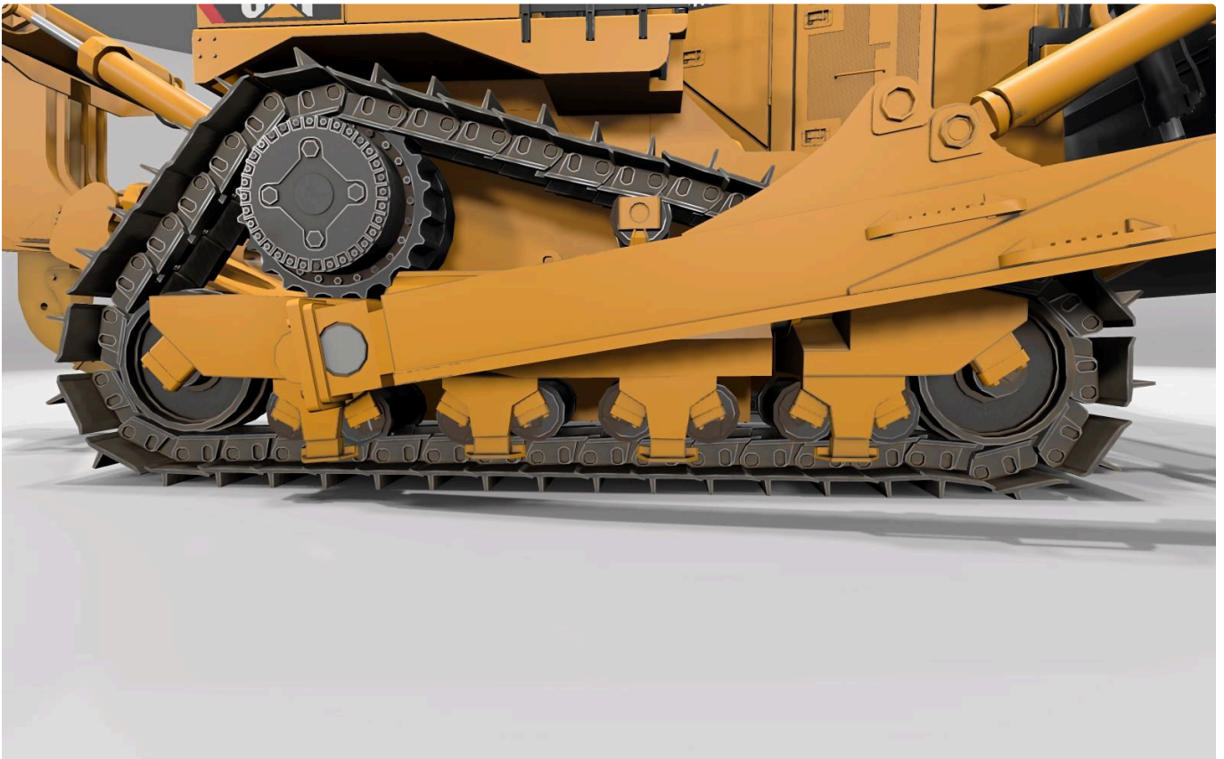
Elevated sprocket, physical track chain, rollers and bogies
