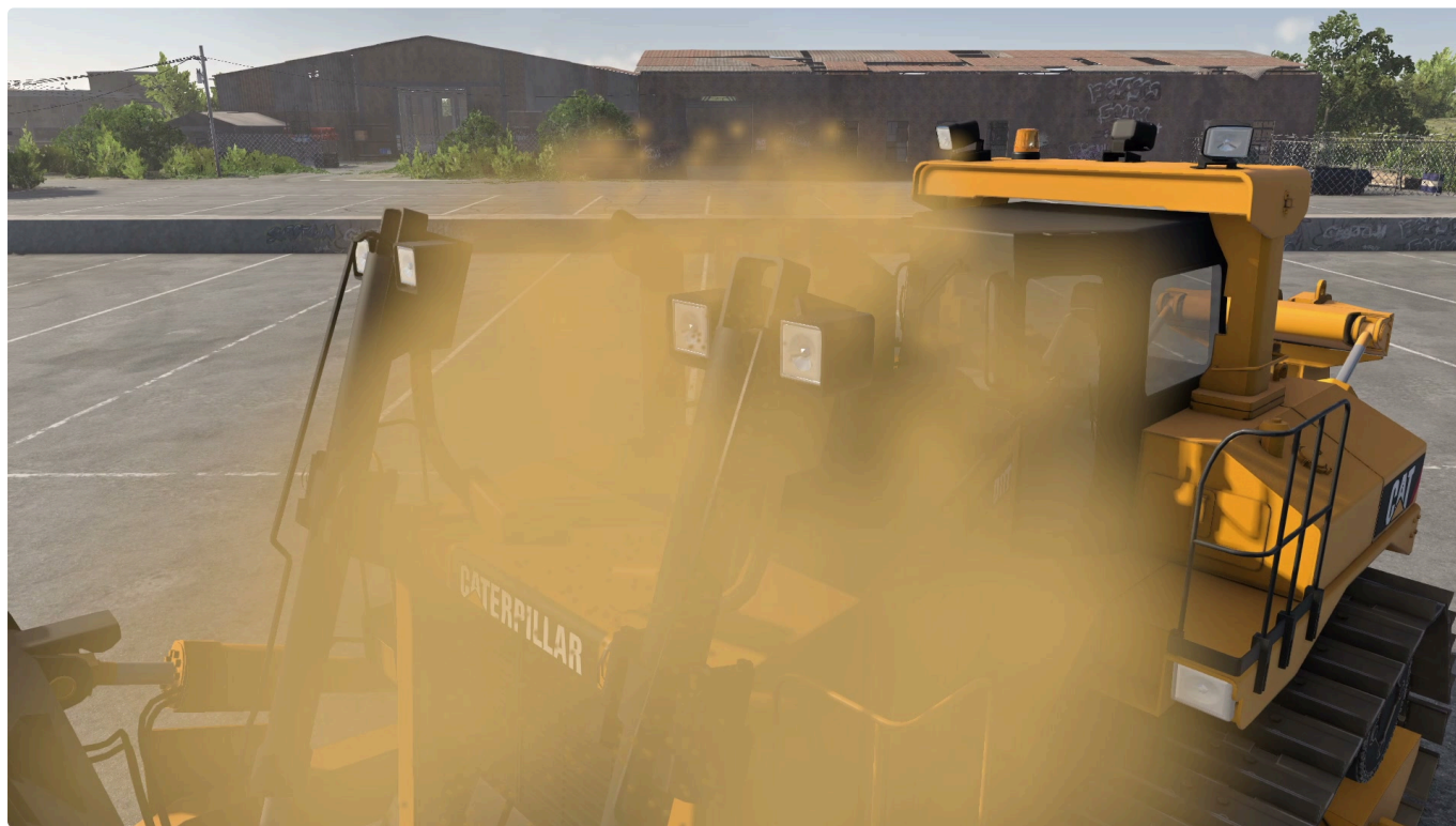
A torn blade-lift line sprays hydraulic oil
