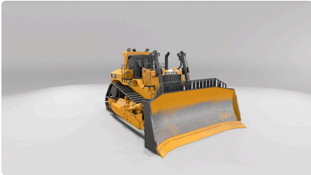
Push Dozer (No Ripper)
