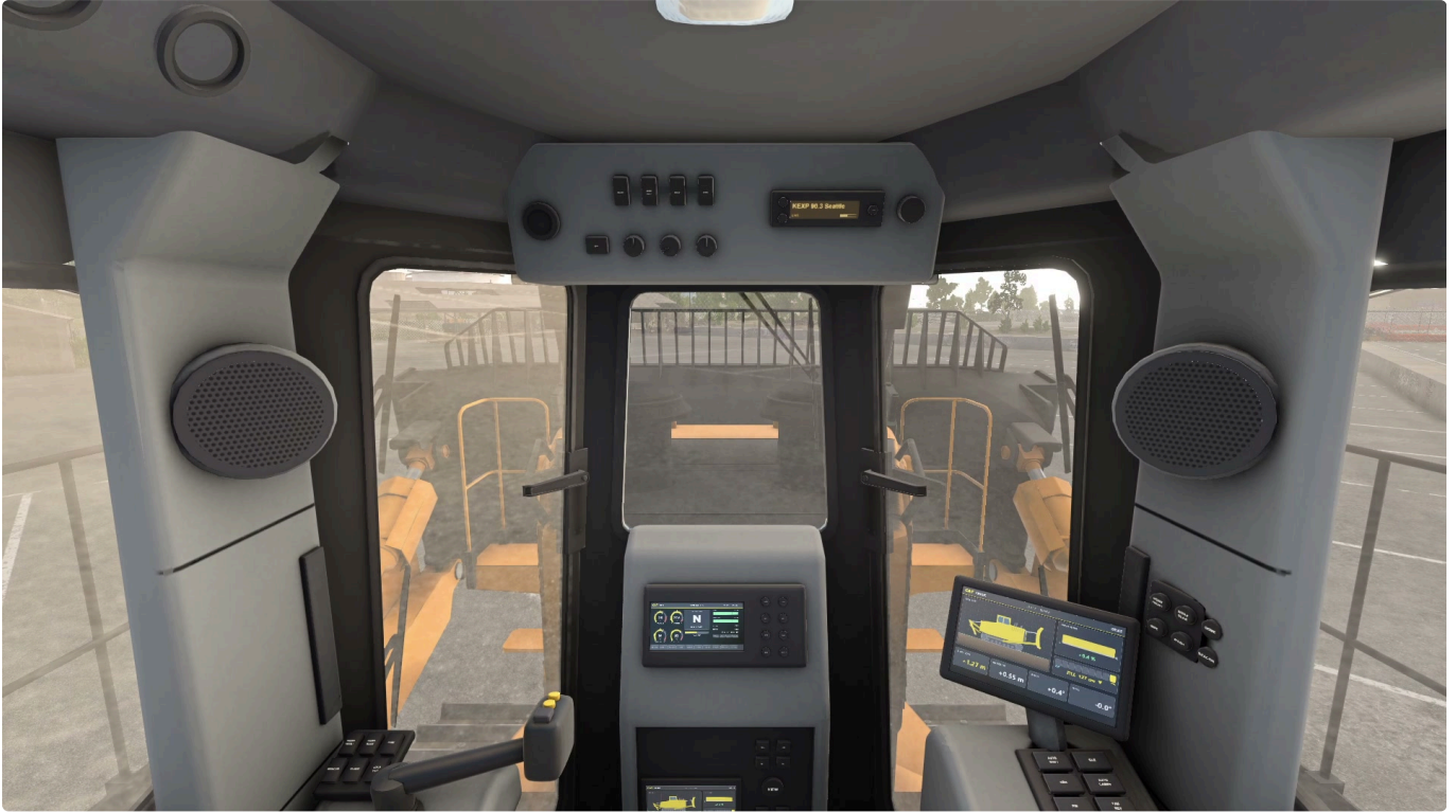
Key on: the operator monitor and grade screen wake up
