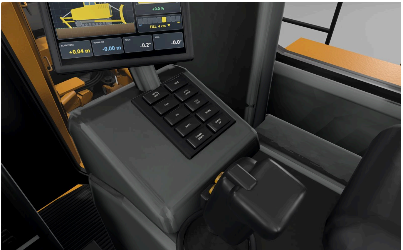
Right console keypad - every function also has a keyboard action
